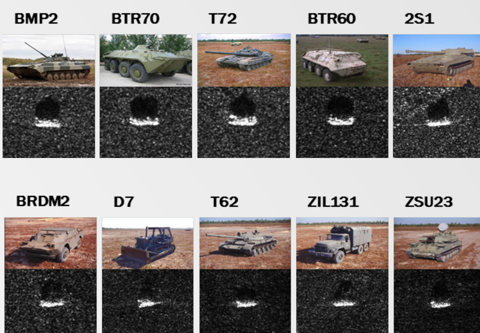
The ten types of vehicles included in the 10-way MSTAR set and examples of their SAR intensity images.
