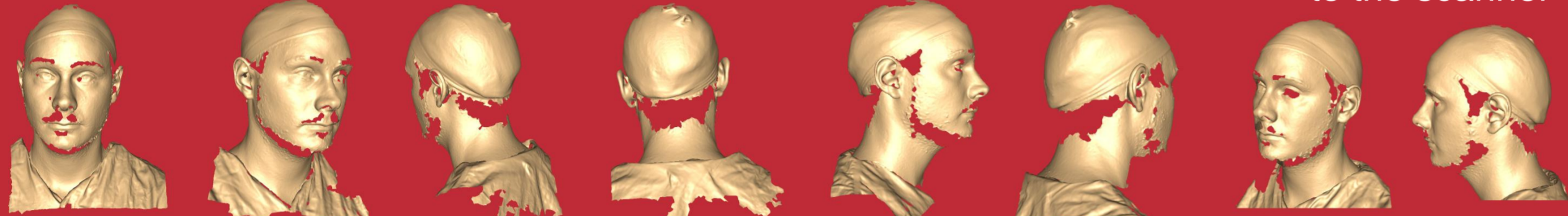
The 8 partial scans captured with the surface scanner
