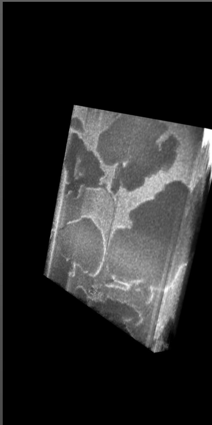
3D image data set with fixed liquid inside of pores
