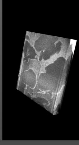
3D image data set with fixed liquid inside of pores
