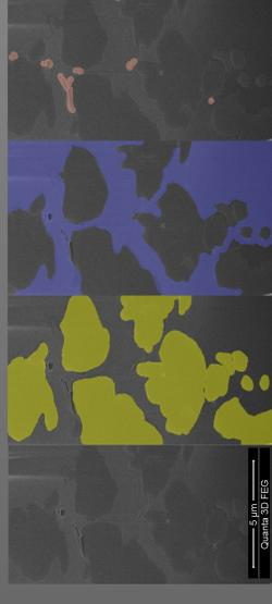
Original image Bulk coloured Pores coloured Air bubbles coloured
