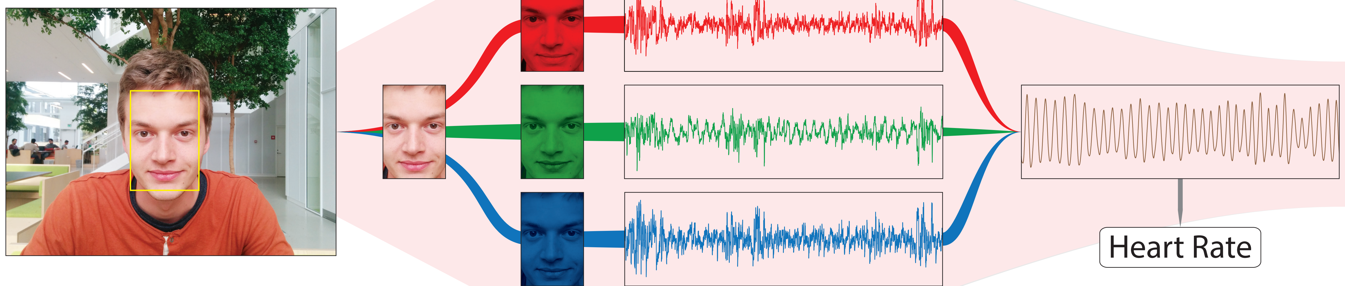
Flow diagram of heart rate estimation
