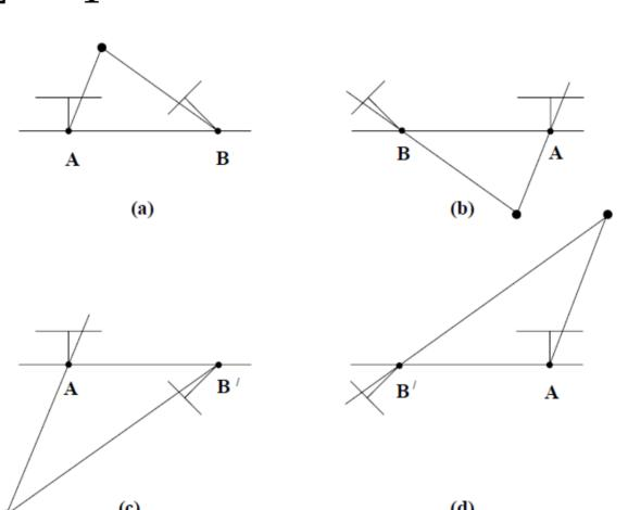
Only one solution has its object in front of both cameras  $\rightarrow$ the robust pairs are triangulated in both camera systems and the sign of the depths is checked, for each possibility. In one case the depths are positive in both systems.
