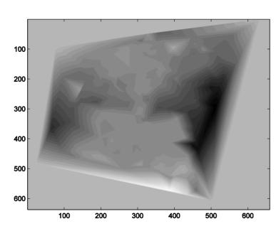
Robust matches are extracted from the rectified images. The rectification error is the vertical distance. A linear interpolation covers the whole bounding geometry.
