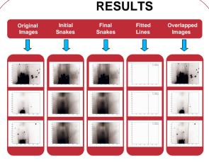
The proposed snake has been tested on a image sequence captured during welding. The results show that the proposed snake can track the edges successfully and continuously. Three frames were selected and shown here.
