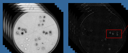
Original multispectral image data and the result of a closing operation on the images. The closing operation is used to bring neighbor pixel information into the pixels. This is done because the mixing model works on a single pixel.
