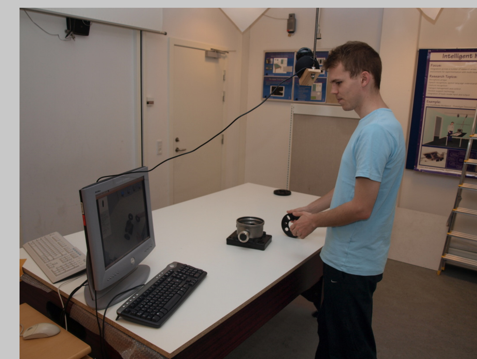
Figure 1: A user is assembling a pump using IAGUAR.
