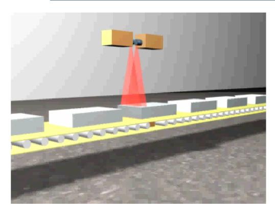
Measurement system consists of two separate x-ray generators and two separate detectors.
